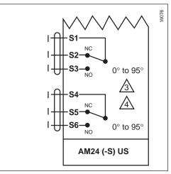
Auxiliary switch wiring for AM24-S US
