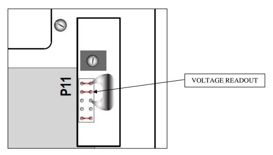
This adjustment ensures that the internal temperature control reset curve starts just as the VFD begins to ramp up. The internal reset signal will be at maximum when the AFB voltage has increased by 6 VDC greater than the minimum volume voltage. If the minimum input voltage is greater than 4 VDC the amount of the internal temperature reset is reduced.
