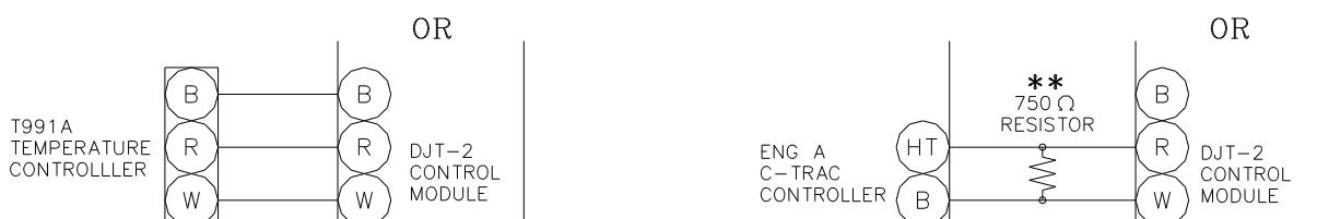
NOTES: 1) OBSERVE POLARITY H TO H AND N TO N IN POWER SUPPLY TO C-TRAC AND DJT-2
