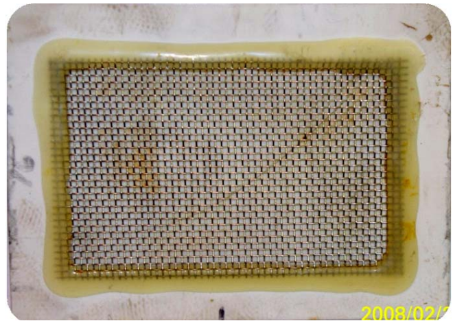
Figure 4: CRACKED CORONA PLATE
