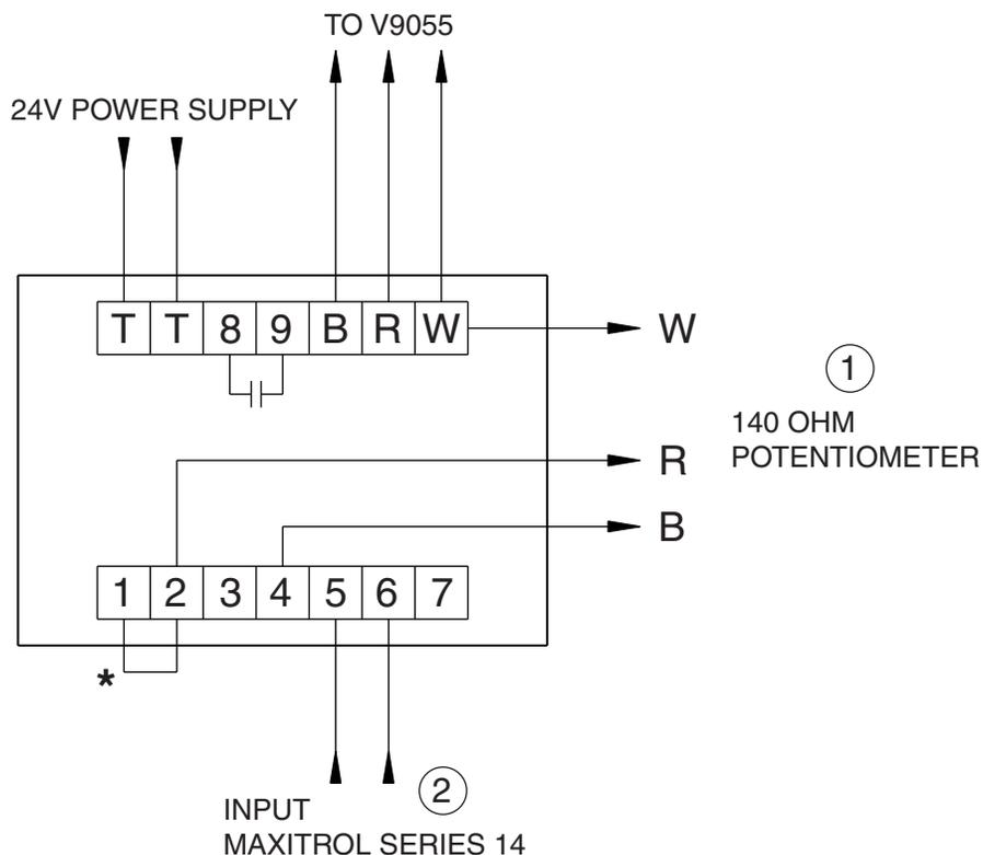
\* NOTE: If using a Maxitrol system on a 109-1, terminals 1 and 2 need to be jumpered.
