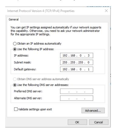
Click OK to accept, and then open a web browser and type in the following address to gain access to the testing interface:
