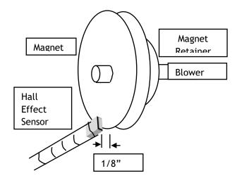
With a digital AC voltmeter, measure the AC volts present on terminals "YS to GS". When the combustion blower is running there should be 4 to 6 Vac present. If the AC voltage is not present, check the tachometer sensor to magnet gap. It should be 1/16 to 1/8 inch. If the gap is satisfactory, attempt to repair by flipping the
